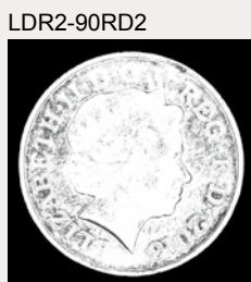
LDR2-90RD2 Edge extraction is difficult with illumination from a high angle.
